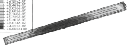
Fig. 8. Simulated deformation cloud chart of thermal stress of optimized turnover beam
