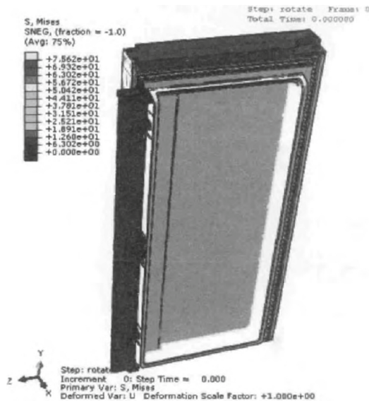
Fig. 5. Simulated stress cloud chart of turning beam
