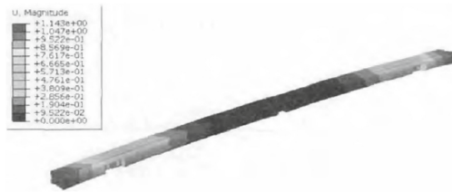
Fig. 4. Cloud chart of thermal stress simulation deformation of turnover beam
