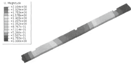
Fig. 3. Simulation deformation cloud chart of turnover beam structure
