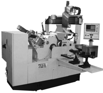
图5 自动上下料装置应用于轴承精密滚子无心磨床 Fig.5 Automatic loading and unloading device for centerless grinder for roller of precision bearing
